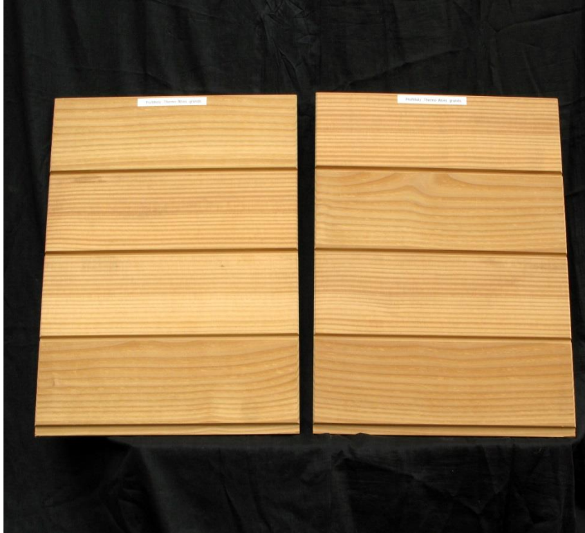
Dado and rabbet joint thermally treated
